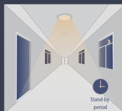
After 5 minutes the light will revert to standby mode and will dim down to 30%
