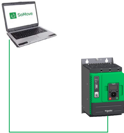
Firmware update through Modbus TCP/Ethernet/IP or Modbus serial using SoMove
