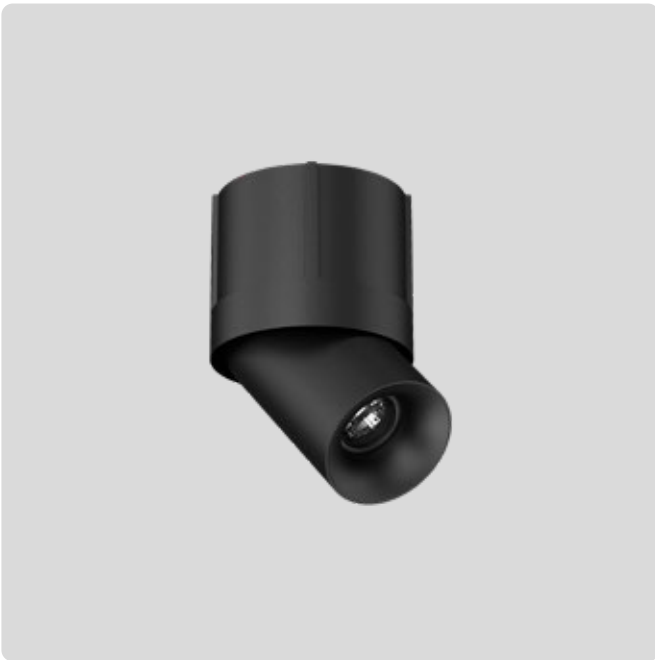
M80-T13 Type 13 - Dark Art Adjustable Spot Watts 12W / 350mA DC Lumens <950lm Beam 45° Tilt/Rotate 40°/355°
