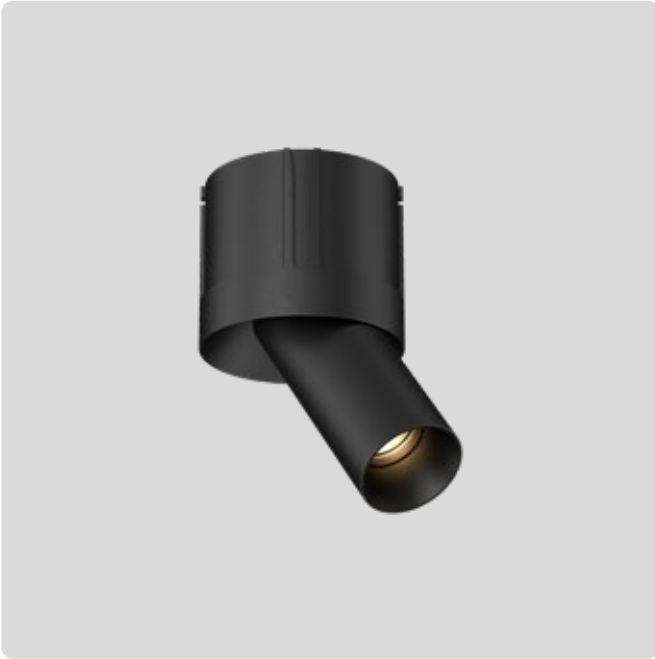
M80-T5 Type 5 - Dark Art Adjustable Spot Watts 9W / 260mA DC Lumens <720lm Beam 36° Tilt/Rotate 38°/355°
