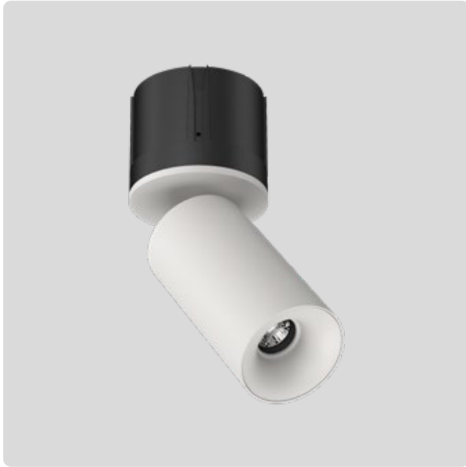
M80-T18 Type 18 - Dark Art Adjustable Spot Watts 9W / 260mA DC Lumens <750lm Beam 45° Tilt/Rotate 90°/355°
