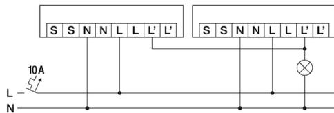
A maximum of 10 devices can be connected in parallel.
