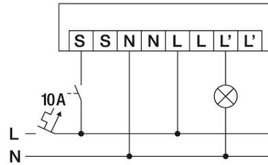
Standard operation with additional control by means of a button
